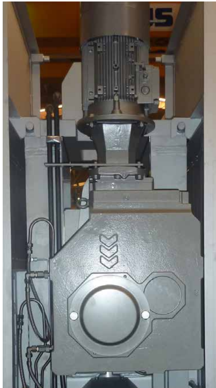
TBR opted for the Watt Drive K139 helical bevel gearbox, mounted on the plant shaft by means of a hollow shaft.
